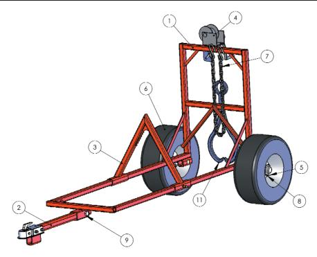
Use the winch and log tong to lift so that you can wrap the chain around the log. Once chain is secure around log - lower the winch so all the weight of the log is on the chain.
