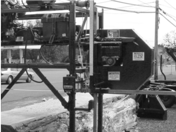
Correct head placement; Operators side is on side with the scale stick and hand winch.
